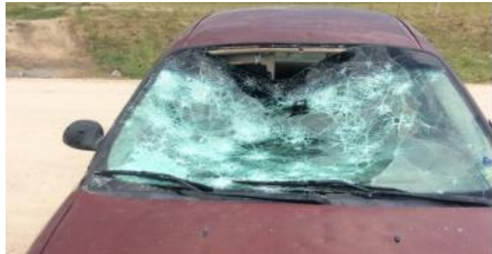
FIGURE 43: JULY 2018 HAIL DAMAGE TO OST VEHICLE
