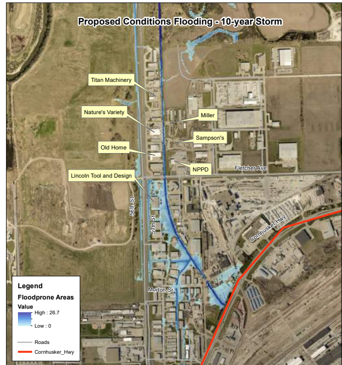
Proposed conditions that reduce floodprone areas
